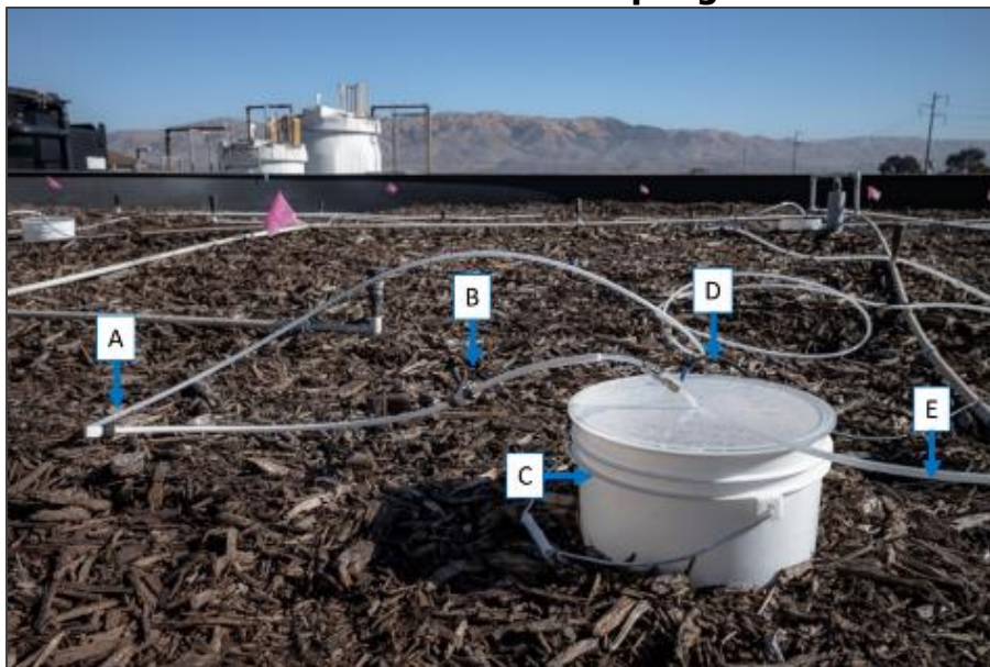
Figure A-39: Surface Flux Chamber for Sampling Biofilter VOC Emissions
