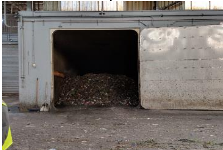
Figure 3: One Anaerobic Digester Bay at ZWEDC After 21-Day Process Completed
