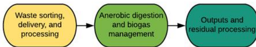
Figure 61: Three Major Anaerobic Digestion (AD) Process Stages
