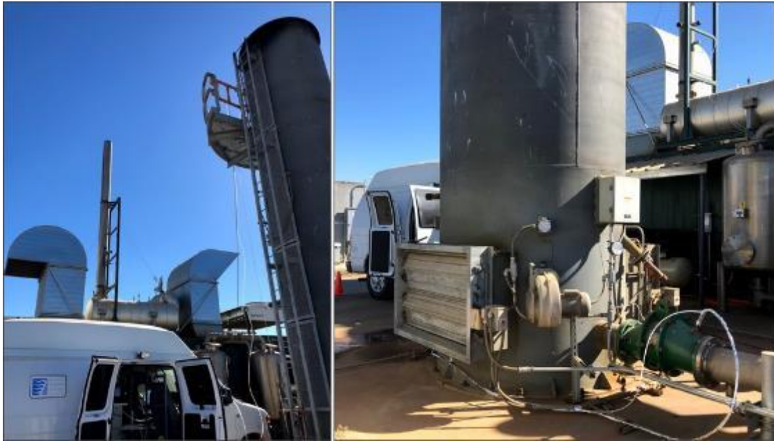
Figure 12: Continuous Sampling Setup at Flare
