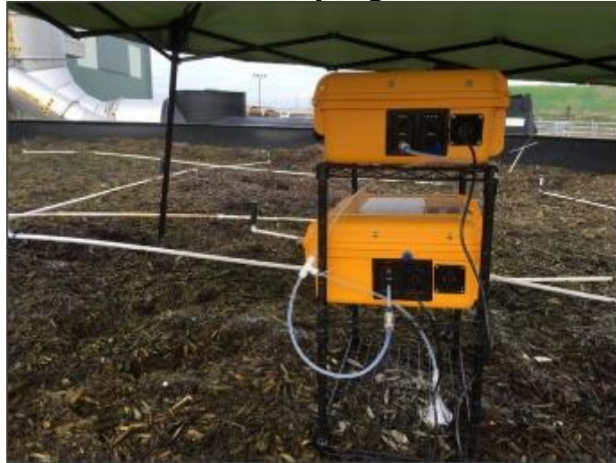
Figure 28: Real-time Sampling on Biofilter Surface
